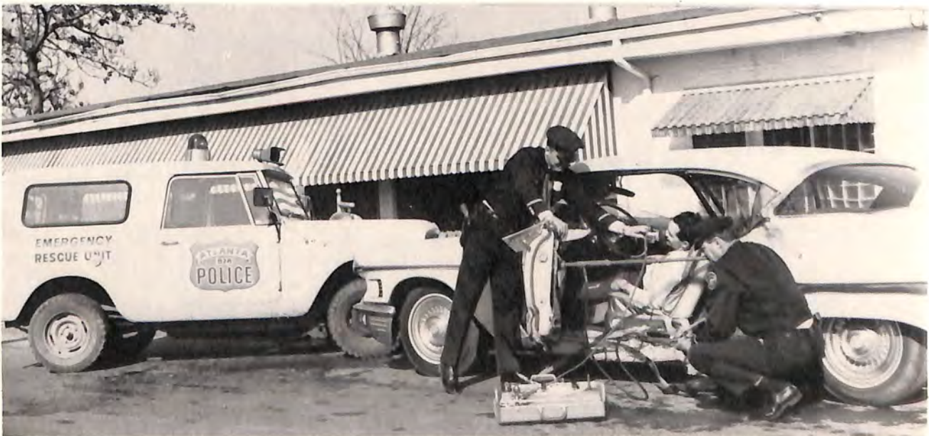
POWER JACK FORCES DOOR OPEN - RESUSCITATOR USED
